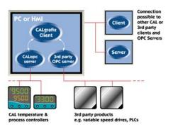
CALgrafix is an OPC (OLE for process control) based software product, which is an open standard for networking process control products. This means ,third party hardware (in this case, a variable speed drive) that has an OPC server can be networked with CAL controllers to create an integrated system.
