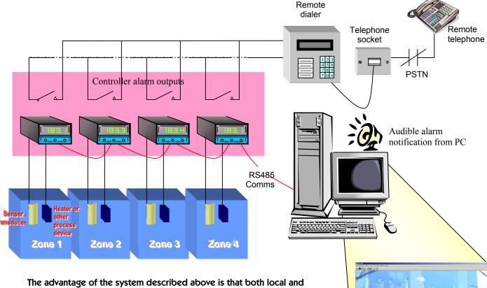
The advantage of the system described above is that both local and remote alarm notification can be configured so that an engineer can be informed of an alarm whether he is on or off-site.
