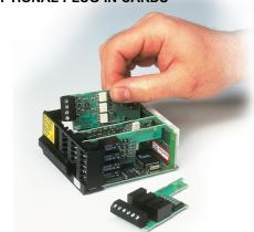
The PAX series meters can be fitted with up to three optional plug-in cards. However, only one card from each function type can be installed at a time. The function types include Setpoint Alarms (PAXCDS), Communications (PAXCDC), and Analog Output (PAXCDL). The cards can be installed initially or at a later date. Each optional plug-in card is shipped with complete installation and programming instructions.
