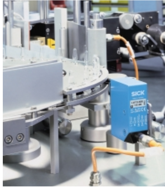
◀ Label present or not: the LUT 3-8 knows the answer (here being used in the pharmaceutical industry).
