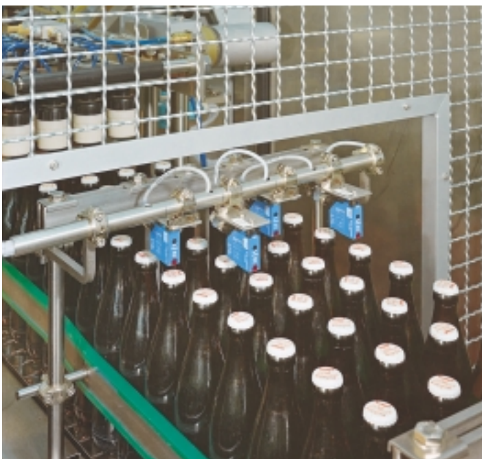
▲ Five-pack instead of six-pack: WT 12-2 photoelectric proximity switches with background suppression detecting gaps in the flow of bottles in an automatic loader.
