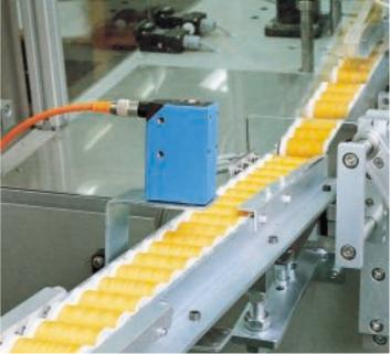
▲ It's the colour that counts: a CS sensor checking the colour of sewing silk before it is packed.
