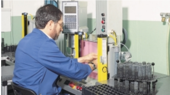
Safeguarding an automatic punch with SICK Light Curtain FGS and one/two cycle mode
