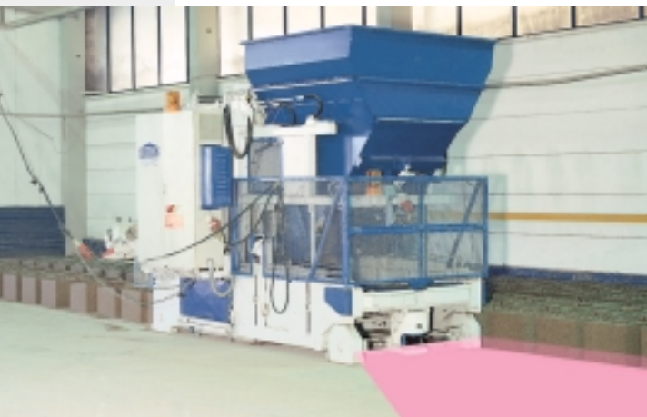
Safeguarding a mobile paving machine with SICK Laser Scanner PLS
