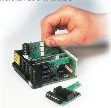
The PAX series meters can be fitted with up to three optional plug-in cards. However, only one card from each function type can be installed at a time. The function types include Setpoint Alarms (PAXCDS), Communications (PAXCDC), and Analog Output (PAXCDL). The cards can be installed initially or at a later date. Each optional plug-in card is shipped with complete installation and programming instructions.
