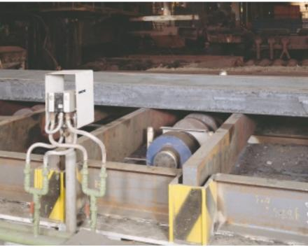
${\color{blue}\blacktriangle}$  Extreme operating conditions exist in steel making plants - the WT 45 photoelectric proximity switch is ideal for many applications, such as detecting metal sheets before they are wound onto coils.
