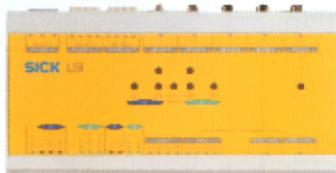
A maximum of four PLS with up to eight warning and protective fields on one or two machines can be controlled by the LSI laser scanner interface. In the case of stationary application, the warning and protective fields are switched by static binary signals, in the case of mobile applications both by static and also dynamic, e.g. speed- and direction-dependent signals.
