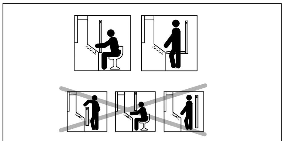
Fig. 2-2: Mounting of the C 2000: Reaching over, under or around the device, or walking behind it, must not be possible.
